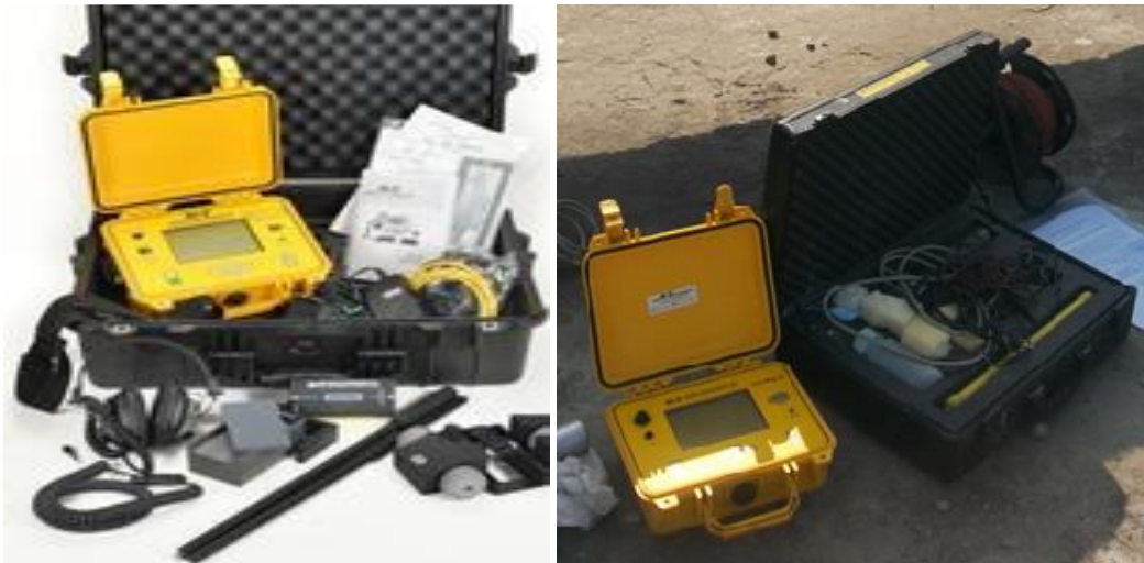
Micro Cover Meter and Half Cell Surveyor
