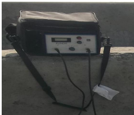
Fig. 3.2: Portable Ultrasound Non destructive Digital Indicator Tester Equipment (PUNDIT)
